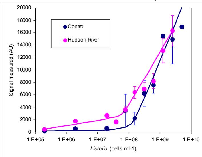
**Figure 2.** Dilutions curves for detection of *Listeria spp* in deionized water (control) and water collected from Hudson River.
